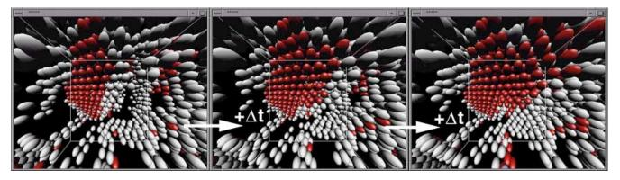
Figure 3. Time animation sequence showing development of stacking faults (red atoms) along Ni grain boundaries
