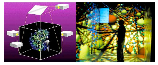
Figure 1. Right image: schematic of a CAVE projection-room showing the location of projectors, Left image: actual snapshot of D\_Atomview in the CAVE running the same data set shown in Figure 8.
