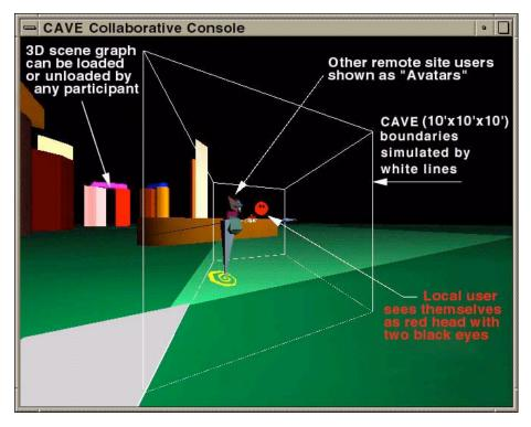
Figure 4. Schematic showing major components of the CAVE Collaborative Console
