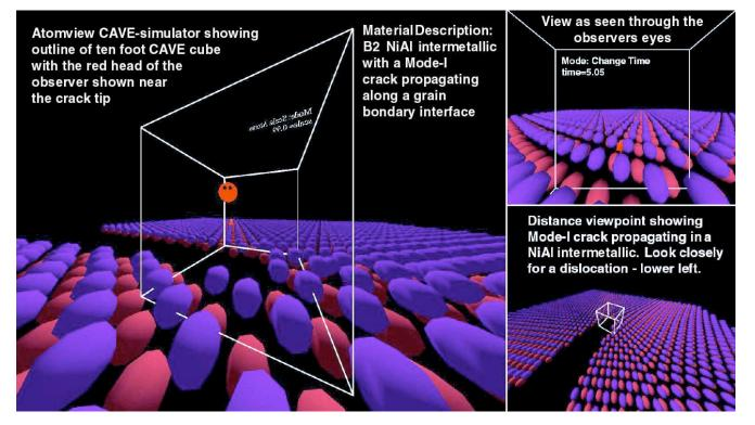
Figure 2. Atomview showing three different views of a B2 NiAL inter-metallic nanostructure as seen by a researcher using a desktop SGI Octane computer viewing HPC results with a CAVE-simulator.
