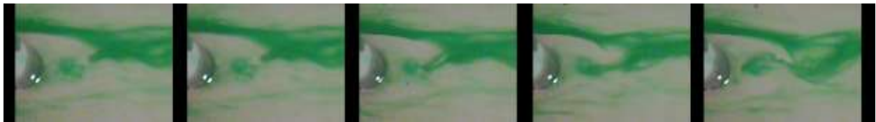
Figure 1.6 Sequence of pictures showing fluid moving backward in the reverse region (M. Ortega 2009)
