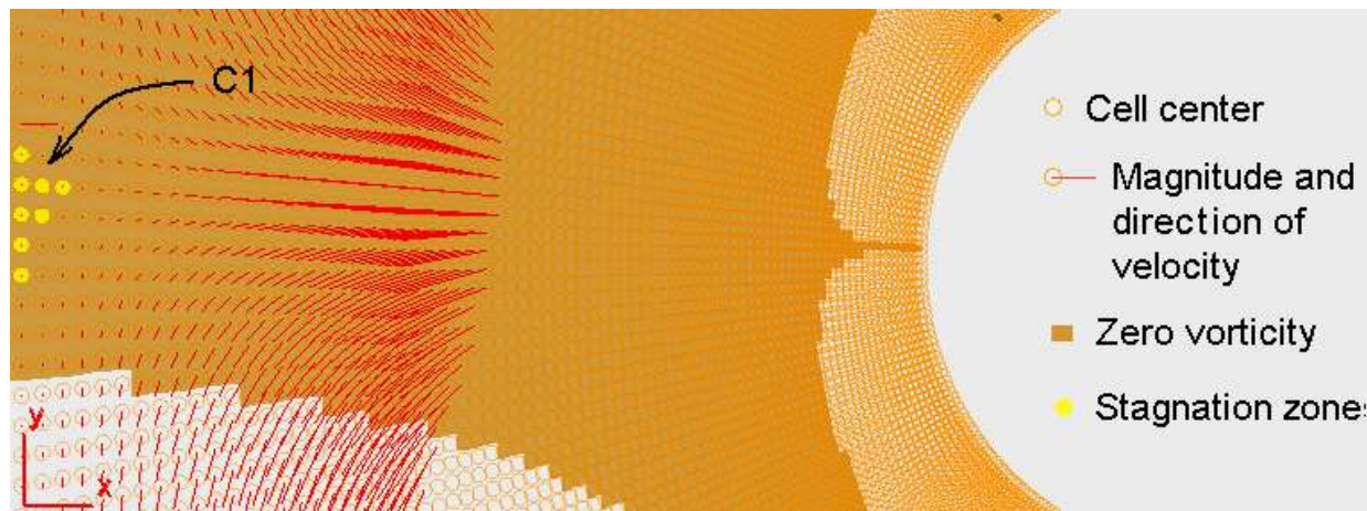
Figure 4.38 Convergence zone C1 at the inlet (moving frame)
