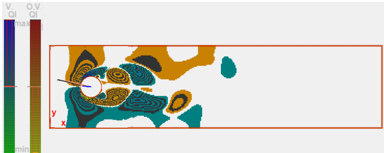
Figure 4.34 Contribution of each point in the domain to the cylinder lift (Min: Yellow, Max: Blue, zero: White)
