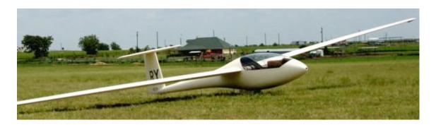
15 Meter with flaps and trailing edge spoilers/dive brakes, Parallelogram stick, Heel brakes, Integrated ballast tanks (115 liters) Competition sealed, Tost CG and nose releases, In-flight adjustable rudders and seat back, Press-to-set trim. Panel: ASI, Compensated 1.2 sec Variometer with audio, Compensated 1.7 sec Variometer with 9v backup power source, Altimeter, Averager, Speed-to-fly calculator, Compass, Oxygen regulator, Voltmeter, 720 Channel transceiver w/Boom mike
